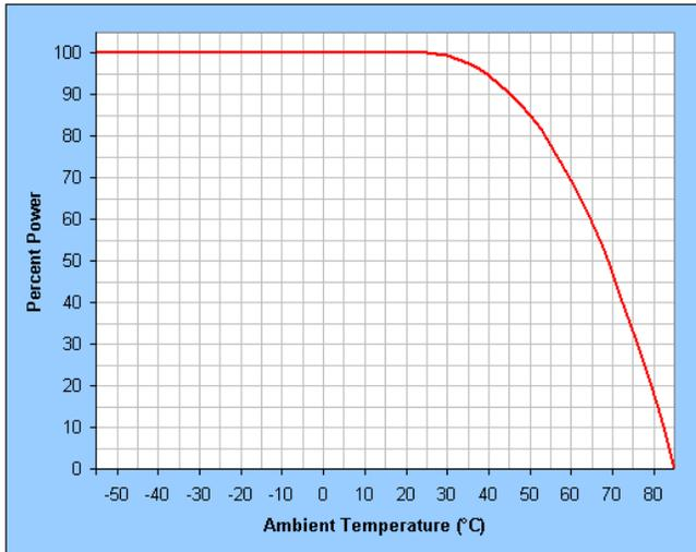
Derating curve for High Energy Ceramic Capacitors.
