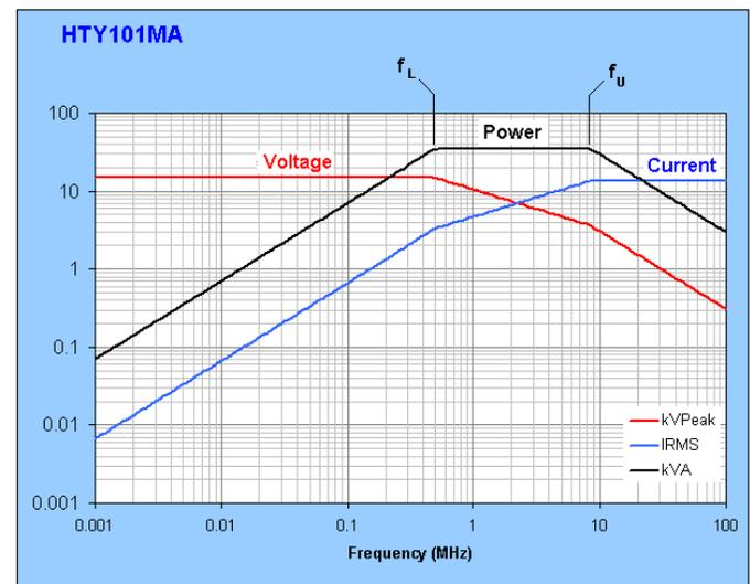
Typical Maximum Rating curves for a ceramic capacitor.
