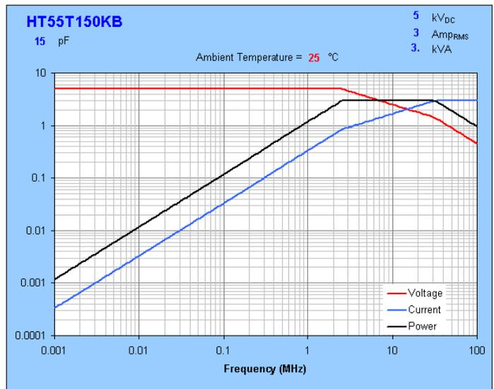
**SPHT Series Ceramic Capacitors** are Class 1 parts featuring high Voltage, Current and Power ratings and low self-inductance. A broad variety of these ‘Power-Disk’ capacitors are offered including the innovative and cost effective ‘Ferris-Wheel’ configuration. All SPHT capacitors have low dissipation factors. Their structure is both simple and robust, assuring a long trouble free life. SPHT Series feature a phenolic resin coating and a long flashover path.
