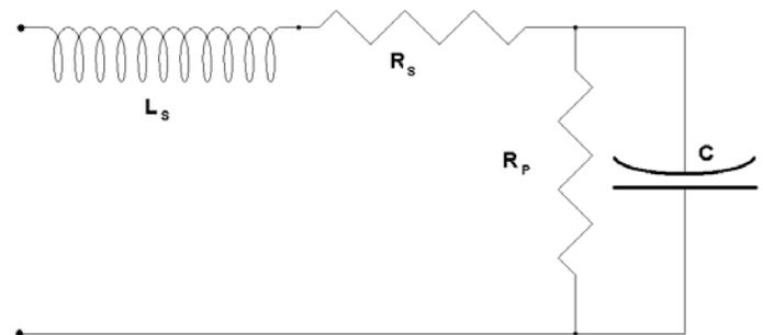
**Equivalent circuit model for a ceramic capacitor.**
