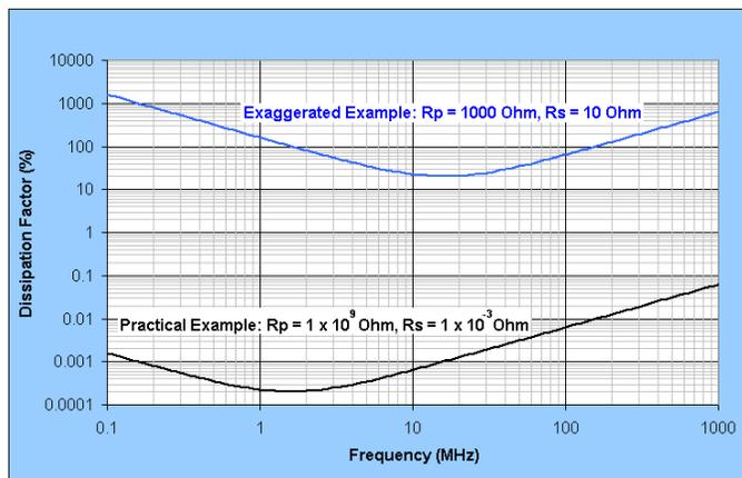
Dissipation Factors comparing effect of  $R_p$  and  $R_s$ .
